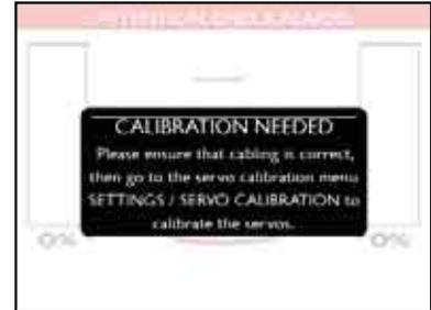
Do not proceed to operate the system until all servos have been successfully calibrated.
